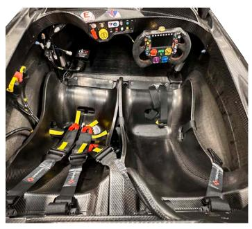
Effortlessly control features such as the lap timer, temperature gauges, car-to-pit radio, and pitlane speed limiter using intuitively-positioned switches directly on the steering wheel.
